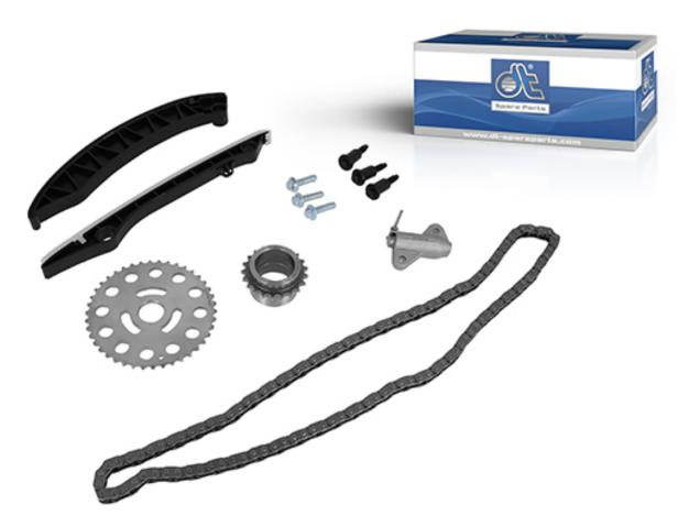
The timing chain is located at the front of the engine and is mounted on two sprockets – on the crankshaft and on the camshaft. The timing chain transmits the rotary motion of the crankshaft to the camshaft, which ensures that the valves open and close at the right time.
