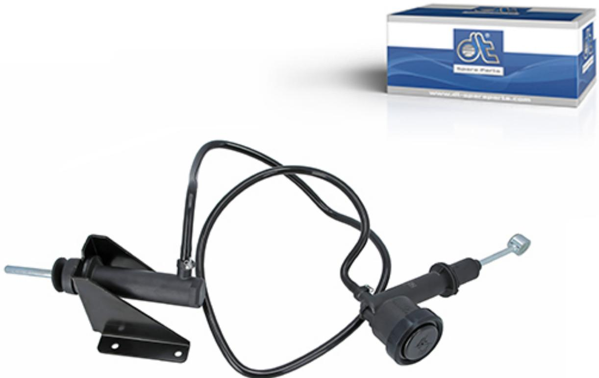
When the clutch pedal is operated, the movement of the piston causes pressure to build up in the clutch master cylinder, which is passed through the hydraulic line to the slave cylinder. From here, the pressure is relayed to the release mechanism, which opens the clutch and thus breaks the flow of power from the engine to the transmission.
