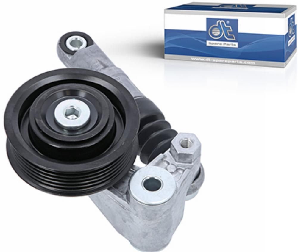
Belt tensioners guide and redirect the belt, ensure the correct tensioning of the V-belt or V-ribbed belt as well as the damping of belt vibrations resulting from changes in load of the motor or the auxiliary units. Furthermore, belt tensioners prevent the belt from severely vibrating where the tightening lengths are long (free, not overlying section of the belt). Belt tensioners and their components are heat-resistant and can withstand high mechanical loads.
