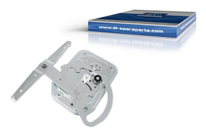
Window regulators are used for lifting and lowering of windows and enable these to be held in any position. In older vehicles, mechanical window regulators are installed and these are operated by a window crank. In new vehicles, powered window regulators are increasingly used, which are operated by an electric motor. The window regulators are individually operated by a switch on the cabin panel.
