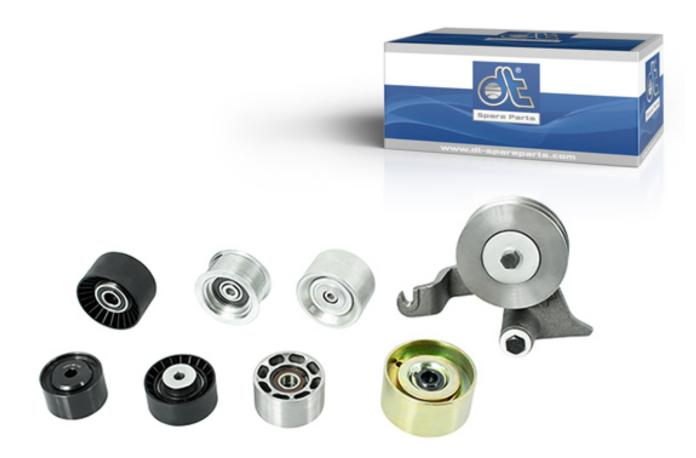
Tensioner pulleys provide precise guidance and constant belt tension in the belt drive. They can either be mounted rigidly or combined with the tensioning elements to belt tensioners. Tensioner pulleys increase the wrap angle on belt drives and thereby transmit higher performance. They enable a change in the rotational direction of the connected aggregates. In combination with belt tensioners, they also compensate for operational belt stretching.
