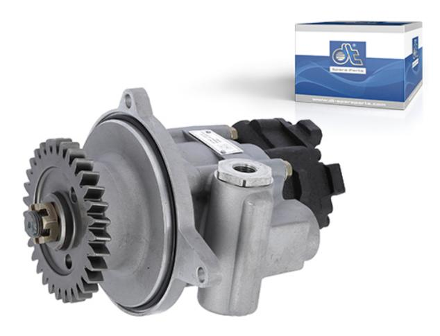
The 2.53183 power steering pump generates the hydraulic oil required for easy steering of the vehicle and supplies it to the steering gear. The integrated gear ensures that the drive runs smoothly and the connected tandem-design fuel pump delivers the fuel from the tank to the injection pump.
