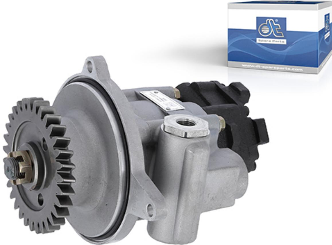
The 2.53183 power steering pump generates the hydraulic oil required for easy steering of the vehicle and supplies it to the steering gear. The integrated gear ensures that the drive runs smoothly and the connected tandem-design fuel pump delivers the fuel from the tank to the injection pump.
