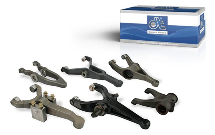
The release fork is a central element of the clutch system. It is connected on one side with the push rod of the clutch slave cylinder and with the release bearing on the other side.
