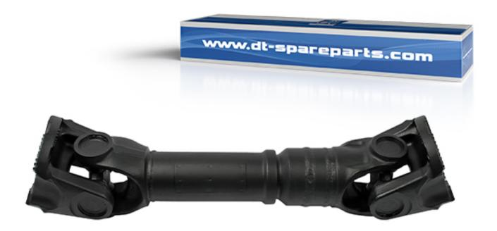
The propeller shaft, also known as the cardan shaft, is an important component in rear-wheel and all-wheel drive. It's job is to transfer the torque in a buckled drive train from the engine or transmission unit to the axle differential. The drive shaft has universal joints so that the motor and axle are not rigidly connected without suspension. It thus ensures mobility during normal driving and compensates for differences in height.
