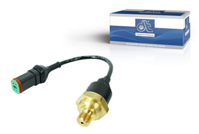
In modern trucks and buses, oil pressure sensors monitor the oil pressure in the motor oil and transmission oil circuit. The measured pressures are recorded in real time in the control unit of the vehicle, evaluated and used to optimise engine parameters. The result is fuel-saving, low emission and more efficient engine operation.
