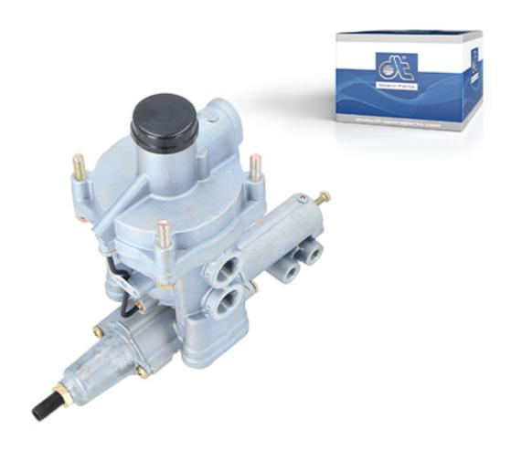
The automatic load-dependent brake force regulator has the task of making the braking effect of a truck dependent on the load condition of the vehicle. With a heavy load, the brakes are applied more and with less load, the braking effect is reduced. This decreases unnecessary wear and prevents the wheels from locking.
