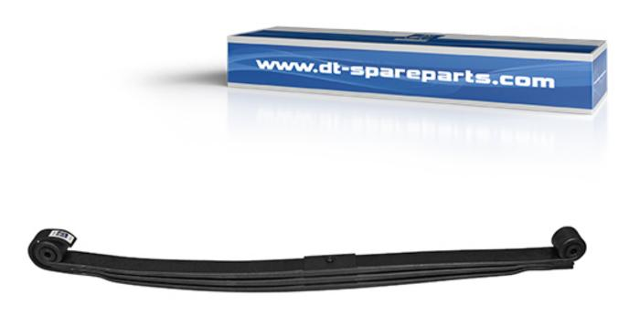
The 4.67601 leaf spring is inserted bilaterally and consists of a flat, arch-tensed profile. Leaf springs are generally among the most important, bend-loaded springs and are most frequently used in air-sprung lorry solid axles and also take on the task of wheel guidance. The leaves consist of several layers, whereby an inherent damping occurs as a result of the friction in the spring. They are attached using centre bolts, spring clamping collar and hinged baseplates.
