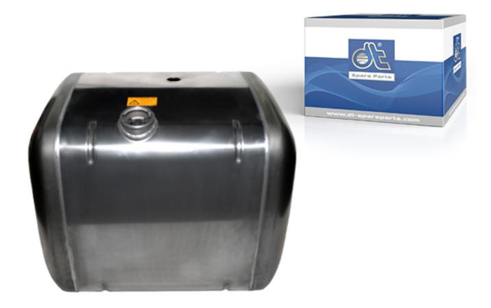
The diesel required to operate the engine is stored in the fuel tank. To save weight, the tank is made of aluminium and in the case of 4.68877, has a volume of 400 litres. It is refuelled via a filler neck and has a vent valve through which trapped and excess air can escape.
