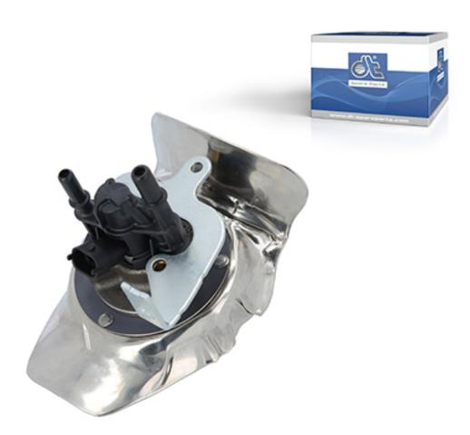
As an important component of the exhaust gas cleaning system, which makes it possible for nitrogen oxide emissions to be reduced by up to 90%, the dosing module individually injects the water-urea mixture in compressed form into the exhaust system. The quantity that is injected depends on the engine speed and vehicle load.
