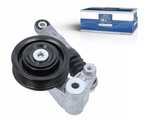
Belt tensioners guide and redirect the belt, ensure the correct tensioning of the V-belt or V-ribbed belt as well as the damping of belt vibrations resulting from changes in load of the motor or the auxiliary units. Furthermore, belt tensioners prevent the belt from severely vibrating where the tightening lengths are long (free, not overlying section of the belt). Belt tensioners and their components are heat-resistant and can withstand high mechanical loads.
