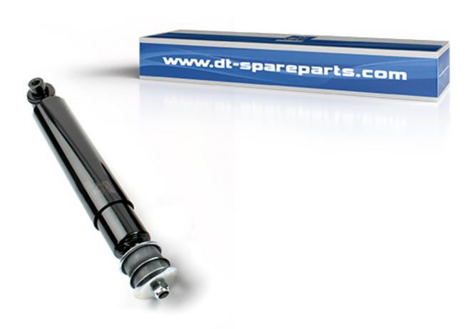
Axle shock absorbers are of great importance for driving safety. They serve to suppress the vibration of the unsprung mass of the vehicle. The impact of shocks which are transmitted to the vehicle by uneven road surfaces is dampened by the shock absorbers. When deciding on the parameters for the level of damping, the best possible compromise is looked for between comfort (low damping force) and driving safety (high damping force).
