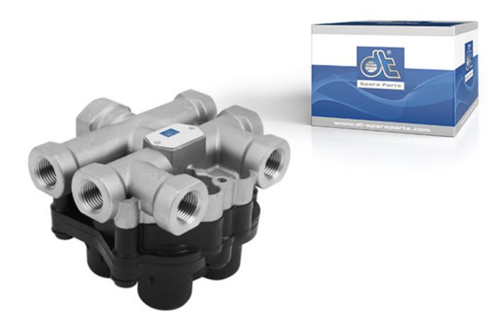
The 4-circuit protection valve isolates the individual circuits of the air pressure braking system from each other.
