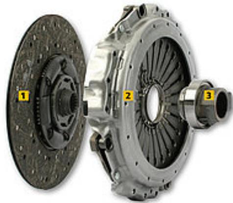
When the clutch rotates, the ball bearing found in the head of the clutch release bearing runs permanently, whereby a preload produced by the control system ensures that the membrane spring tongue and ring guide in the clutch release bearing run at the same speed.
