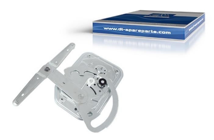
Window regulators are used for lifting and lowering of windows and enable these to be held in any position. In older vehicles, mechanical window regulators are installed and these are operated by a window crank. In new vehicles, powered window regulators are increasingly used, which are operated by an electric motor. The window regulators are individually operated by a switch on the cabin panel.
