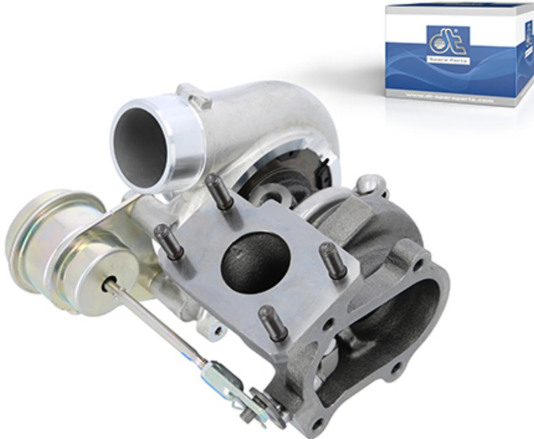
Exhaust turbochargers consist of two flow machines; one turbine and one compressor that are placed on a joint shaft. The compressor draws in fresh air, which is then pressed through the charging air cooler for cooling down and then up to 2 bar in the combustion chamber.
