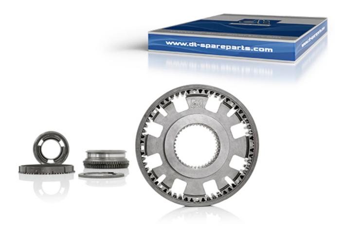
Synchronizer gears form the transition between gearwheel and shift collar. Through friction, they bring both wheels of the required gear to the same rotational speed, so that this can be engaged without declutching.
