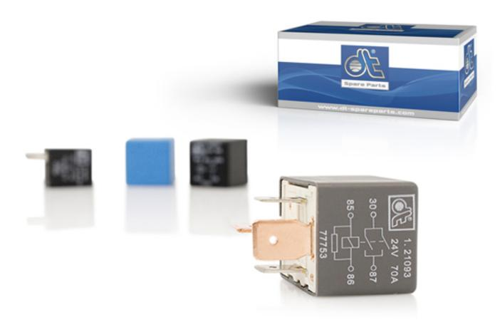
Relays are used to separate electrical circuits and to switch electrical consumers up to a current of 70 amperes. The advantages of relays are the compact design and the possibility of switching large electrical consumers with low currents. Furthermore, relays provide the possibility of switching higher voltages with low control voltages.
