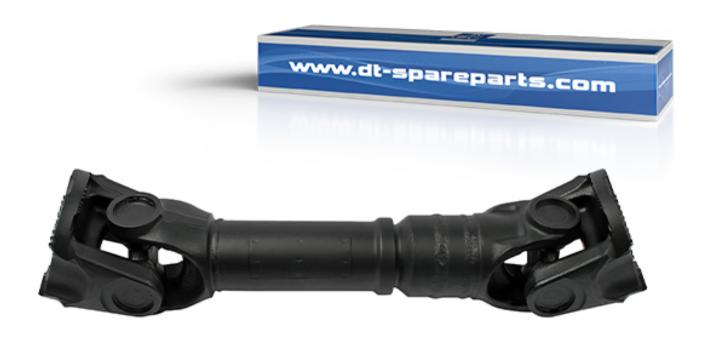
The propeller shaft, also known as the cardan shaft, is an important component in rear-wheel and all-wheel drive. It's job is to transfer the torque in a buckled drive train from the engine or transmission unit to the axle differential. The drive shaft has universal joints so that the motor and axle are not rigidly connected without suspension. It thus ensures mobility during normal driving and compensates for differences in height.
