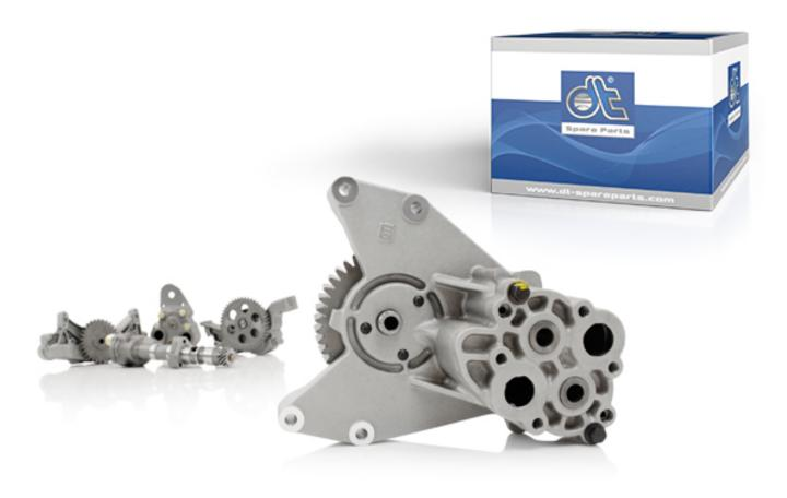
The oil pump is an essential part of the engine lubrication system. The main purpose of engine lubrication is to reduce friction between gliding components, which results in a reduction in wear. Oil is sucked by the oil pump from the sump, pumped through filter and cooler, and finally conveyed through pipes and channels to the lubrication points.
