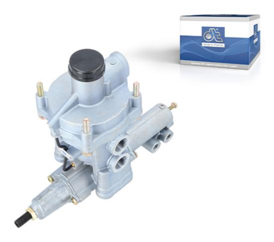
The automatic load-dependent brake force regulator has the task of making the braking effect of a truck dependent on the load condition of the vehicle. With a heavy load, the brakes are applied more and with less load, the braking effect is reduced. This decreases unnecessary wear and prevents the wheels from locking.
