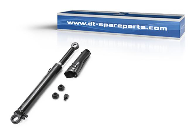
DT® brand hydraulic cylinders consist of a tube with precisely toleranced dimensions, a hard-chrome plated piston rod with very low roughness and high level of hardness as protection against corrosion, as well as a bolted or welded mounting eye or fork. Protection against corrosion of the fixing bolt is ensured by mounted sealing rings.
