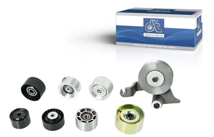
Tensioner pulleys provide precise guidance and constant belt tension in the belt drive. They can either be mounted rigidly or combined with the tensioning elements to belt tensioners. Tensioner pulleys increase the wrap angle on belt drives and thereby transmit higher performance. They enable a change in the rotational direction of the connected aggregates. In combination with belt tensioners, they also compensate for operational belt stretching.
