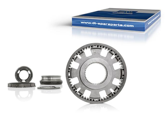
Synchronizer gears form the transition between gearwheel and shift collar. Through friction, they bring both wheels of the required gear to the same rotational speed, so that this can be engaged without declutching.
