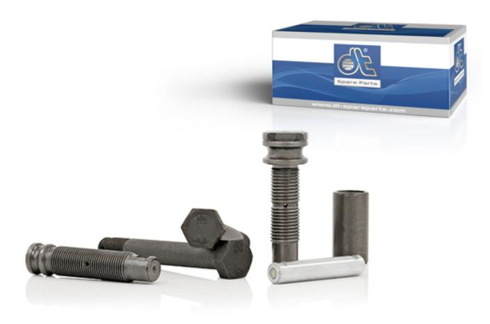
Spring bolts are safety-relevant components and, together with the spring bushing, are used to connect axle springs and frame holder. The high-strength connecting elements are available in various geometric forms, according to the application, area of use and the requirements. Depending on the construction of the axle spring and the corresponding spring bushing, different types are used.
