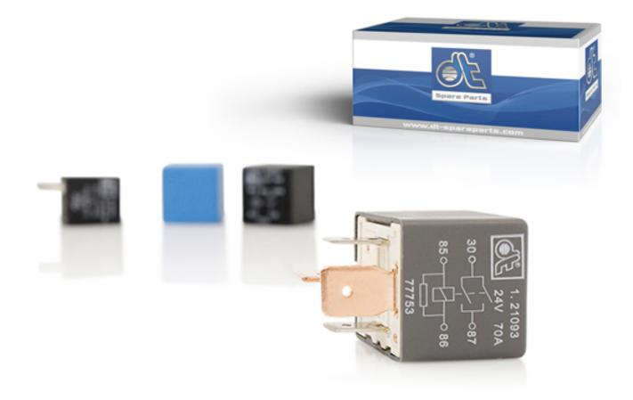
Relays are used to separate electrical circuits and to switch electrical consumers up to a current of 70 amperes. The advantages of relays are the compact design and the possibility of switching large electrical consumers with low currents. Furthermore, relays provide the possibility of switching higher voltages with low control voltages.
