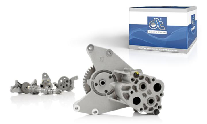
The oil pump is an essential part of the engine lubrication system. The main purpose of engine lubrication is to reduce friction between gliding components, which results in a reduction in wear. Oil is sucked by the oil pump from the sump, pumped through filter and cooler, and finally conveyed through pipes and channels to the lubrication points.
