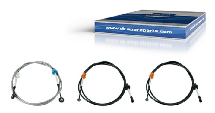
Gearshift cables transmit forces from the gear shift lever to the transmission. As soon as a gear is selected or changed by the driver, the gearshift cable transmits this mechanical impulse to the transmission. Tensile forces of up to 7 kilo Newton are transmitted over distances of sometimes up to more than 4 metres.
