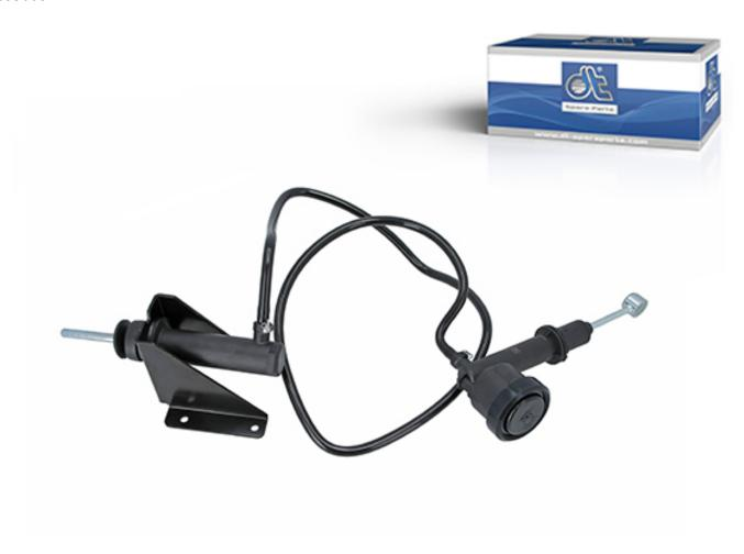
When the clutch pedal is operated, the movement of the piston causes pressure to build up in the clutch master cylinder, which is passed through the hydraulic line to the slave cylinder. From here, the pressure is relayed to the release mechanism, which opens the clutch and thus breaks the fl ow of power from the engine to the transmission.
