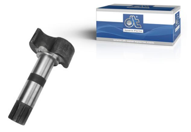
Brake camshafts are used in Simplex drum brakes. They serve to transfer the power generated by the pneumatic brake cylinder, via a slack adjuster, to both brake shoes.
