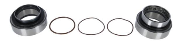
The axles and shafts are supported and guided by the wheel bearings, which means that the wheels turn easily on the axles with little friction. The radial or axial forces of the wheels caused by driving, braking and turning corners are absorbed by the wheel bearings.
